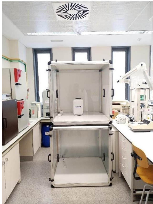
Figure 1: Picture of 1x1x1m cabins used. The cabin on the top was used to make the tests of the WELLISAIR device and the cabin on the bottom was used for CONTROL purpose.
